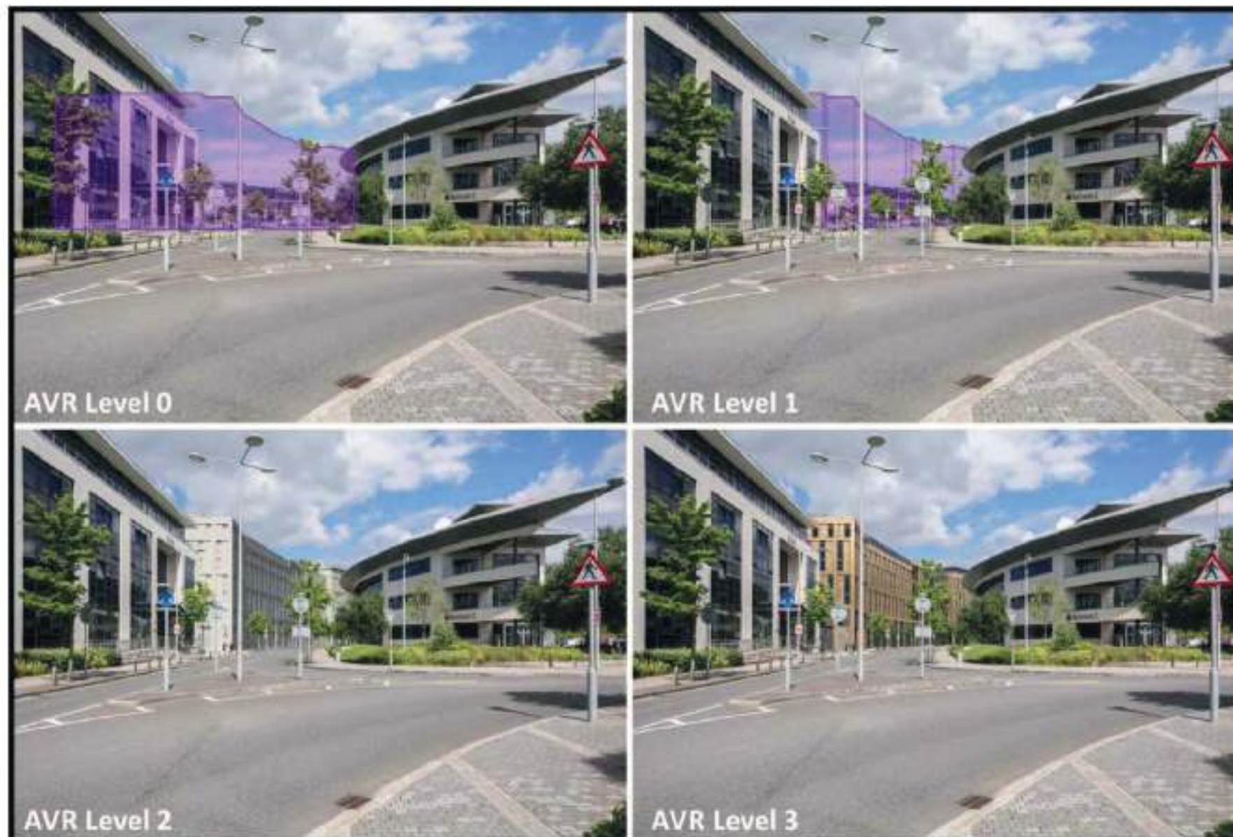
Figure A6-1: Accurate Visual Representation (AVR) Levels 0-3
