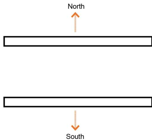
In Passivhaus design teaching spaces to be orientated North or South for optimum control of solar gain
