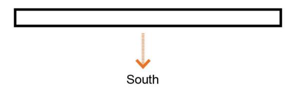
In Passivhaus design teaching spaces to be orientated North or South for optimum control of solar gain
