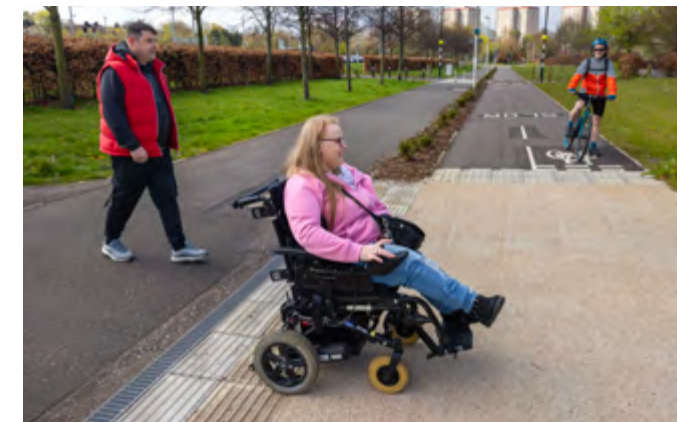
Creating a pleasant, safe and environment for walking and wheeling - Routes must be of appropriate clear width with features like tactile paving to warn users of hazards. © Sustrans.
